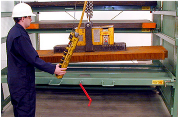
An operator retrieves thick plate out of a Crank-Out Sheet Rack Drawer with magnet lifter
