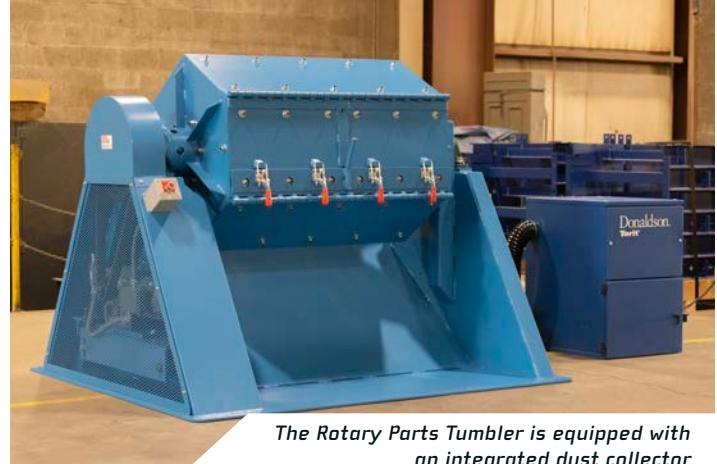
*The Rotary Parts Tumbler is equipped with an integrated dust collector*
