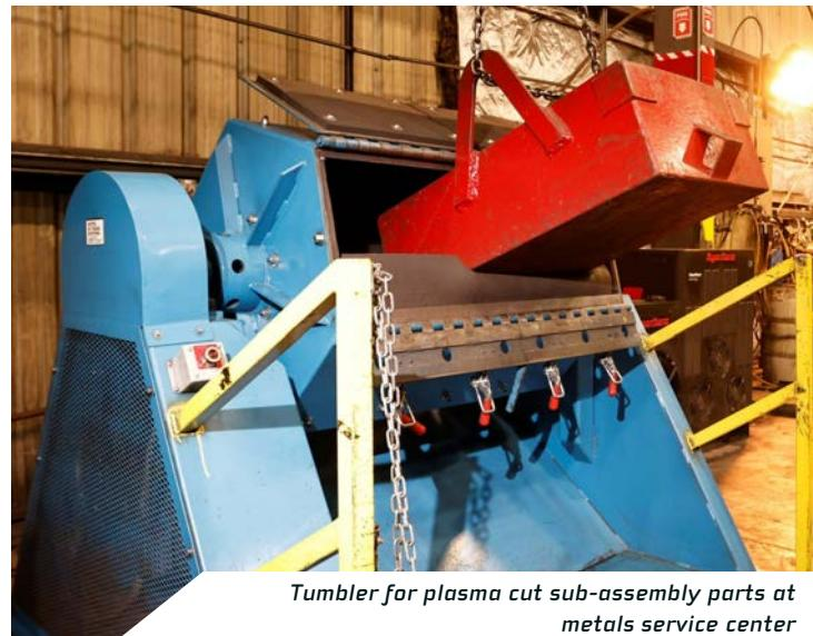
*Tumbler for plasma cut sub-assembly parts at metals service center*
